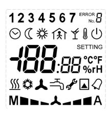
Over Modbus, it is possible to set / reset the complete symbol set except for the 7 segment digits, "Error" and "Setting" texts, and symbols of °C, °F, %, and rH. Those are part of the configurable menu profiles. The register description is available in a separate document *Room units UI... – Communication description*.
