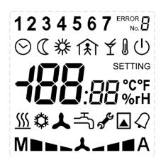
A large (60 x 60 mm) display clearly shows actual room temperature and controller status with 7-segment digits and standard Day, Night, Off, and Time scheduler symbols. Active output is indicated by a heating symbol. In the upper part, there are week days used for time scheduler setup. Other symbols are not used.
