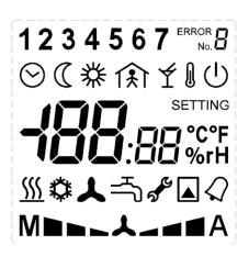
A large (60 x 60 mm) display clearly shows actual room temperature and controller status with 7-segment digits and standard Day, Night, Off, and Time scheduler symbols. Active output is indicated by a heating symbol. In the upper part, there are week days used for time scheduler setup. Other symbols are not used.
