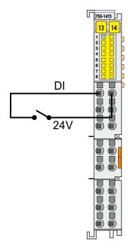
Active state of each input is **indicated** by green LED (on = logical one detected).
