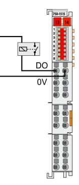
Switched status of each output is indicated by a green LED in the upper part of the module.
