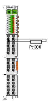
Operational readiness and trouble-free data bus communication of each input is **indicated** by green LED. Red LED indicates wire break, short circuit or signal out of its measuring range.
