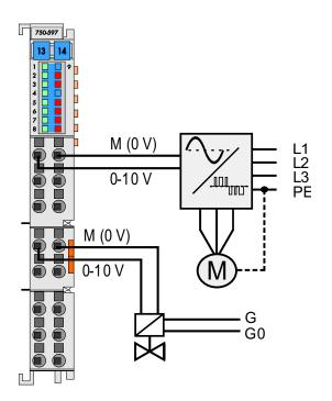
Operational readiness and trouble-free data bus communication of each channel is **indicated** by green LED. Red LED indicates status of the field power suply voltage (undervoltage or general error).
