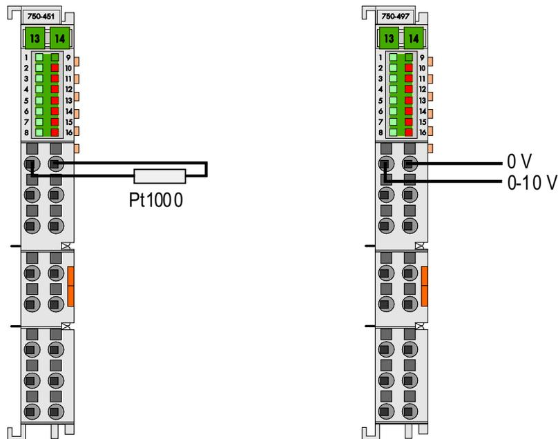
Operational readiness and trouble-free data bus communication of each input is **indicated** by green LED. For the 750-497 module, red LED indicates when measuring range is exceeded or falls below its limit for a given input. For the 750-451 module, red LED indicates wire break, short circuit or when signal is out of measuring range.
