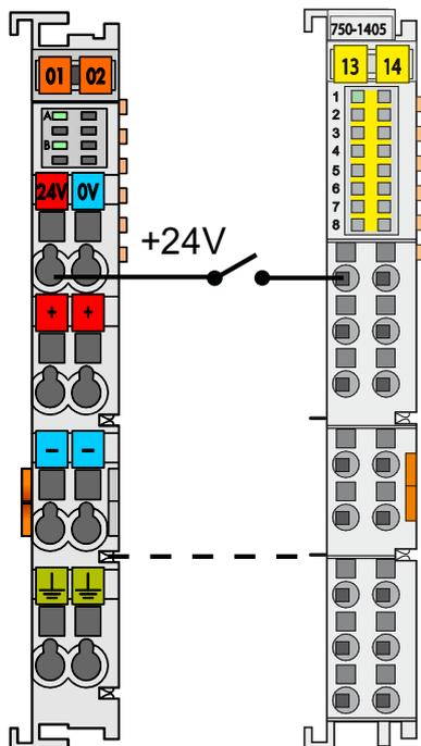
Dashed line is via PLC internal bus.
