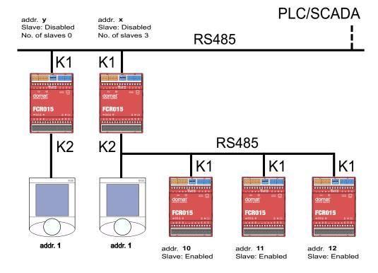
In this connection, controllers with addresses x, 10, 11, and 12 are in one zone and all of them are controlled by one room unit. The room unit must be set to address 1. The controller addressed x is a master. Outputs of controllers addressed 10, 11, and 12 are controlled by the same signals as the master controller addressed x.
