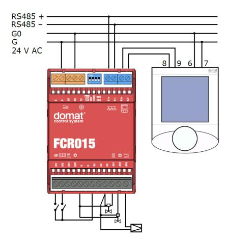
Power supply G and G0 terminals are internally connected with G and G0 terminals on the lower terminals block.
