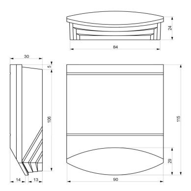
Temperature sensor. Dimensions are in mm.
