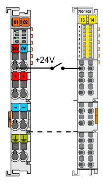
Dashed line is via PLC internal bus.
