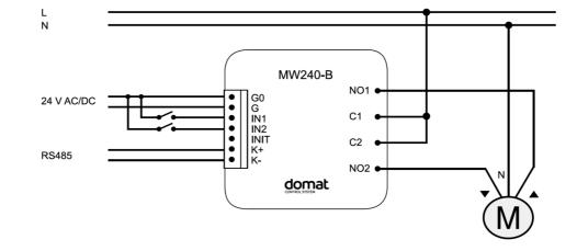
Installation For installation of MW240-B module is recommended to use flat surface or a flushmounting box with minimal inner diameter 65 mm and minimal depth 65 mm.
