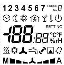
A large ( $60 \times 60$  mm) display clearly shows actual room temperature and controller status with 7-segment digits and standard Day, Night, Off, and Time scheduler symbols. Active output is indicated by a heating symbol. In the upper part, there are weekdays used for time scheduler setup. Other symbols are not used.
