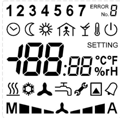
A large (60 × 60 mm) display clearly shows actual room temperature and controller status with 7-segment digits and standard Day, Night, Off, and Time scheduler symbols. Active output is indicated by a heating symbol. In the upper part, there are week days used for time scheduler setup. Other symbols are not used.
