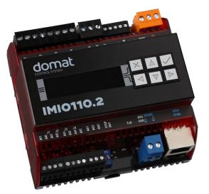
Summary DDC (Direct digital control) controllers IMIO105.2 and IMIO110.2 are free programmable process station with ARM i.MX6UL processor and Linux OS. It contains two Ethernet ports, 4 × AI, 4 × DI, 2 × AO, 6 × DO and RS485 interface. Controllers are suitable for control of larger installations (approximately 400 to 500 physical data points).
