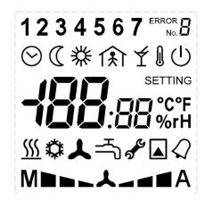
Over Modbus, it is possible to set / reset the complete symbol set except for the 7 segment digits, "Error" and "Setting" texts, and symbols of °C, °F, %, and rH. Those are part of the configurable menu profiles. The register description is available in a separate document *Room units UI...* – *Communication description*.
