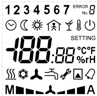
Over Modbus, it is possible to set / reset the complete symbol set except for the 7 segment digits, „Error“ and „Setting“ texts, and symbols of °C, °F, %, and rH. Those are part of the configurable menu profiles. The register description is available in a separate document *Room units UI... – Communication description*.
