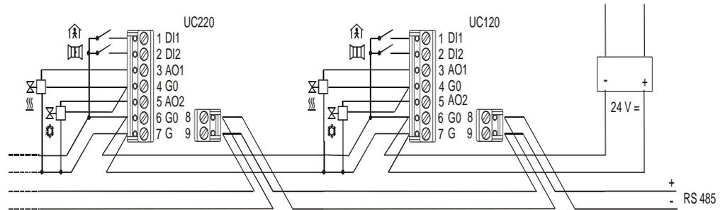
Connection of power and communication. Suitable cable types are LAM DATAPAR 2x0.8 (cross-section in mm<sup>2</sup>), JYTY 2x1 (diameter in mm) etc. If communication and power are in the same cable, use 4-core LAM DATAPAR 2x2x0.8, JYTY 4x1. Up to 100-120 meters, parallel lines of 24 V and data bus are no problem. Regarding to EMC it is better if the pairs are twisted, such as with the LAM DATAPAR or Belden 8205 cable.
