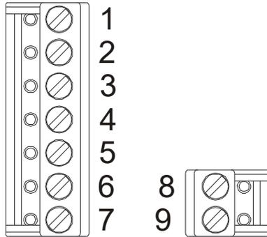
1: DI1 presence input (active when connected to G0)
