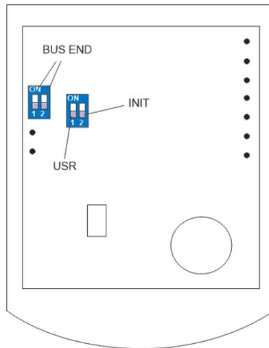
**BUS END:** if ON, the bus is terminated (if last device on the line)
