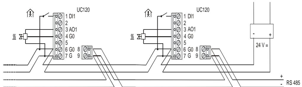
Connection of power, communication, and valve. Suitable cable types are LAM DATAPAR 2x0.8 (cross-section in mm<sup>2</sup>), JYTY 2x1 (diameter in mm) etc. If communication and power are in the same cable, use 4-core LAM DATAPAR 2x2x0.8, JYTY 4x1. Up to 100-120 meters, parallel lines of 24 V and data bus are no problem. Regarding to EMC it is better if the pairs are twisted, such as with the LAM DATAPAR or Belden 8205 cable.
