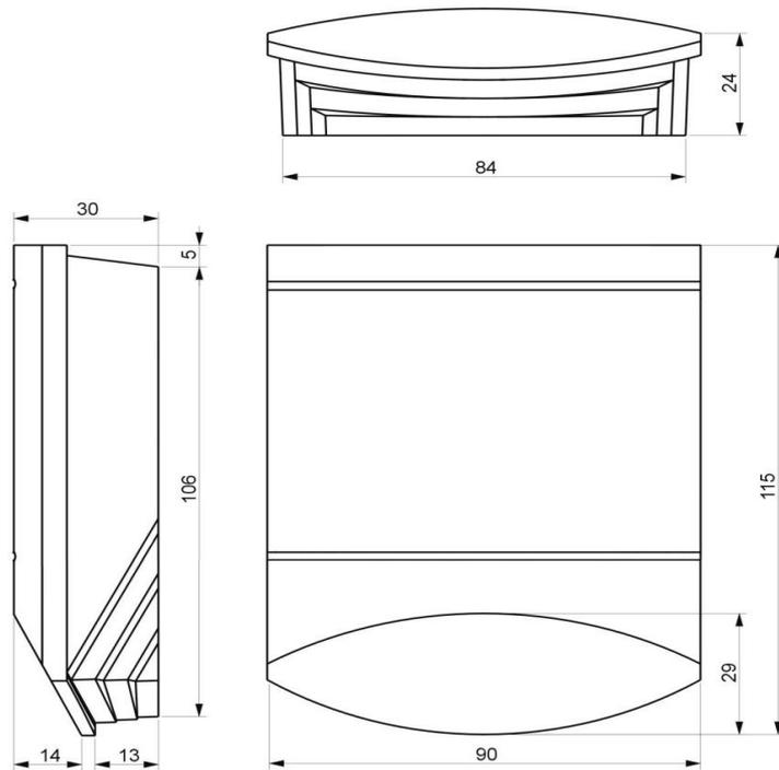
Temperature sensor. Dimensions are in *mm*.
