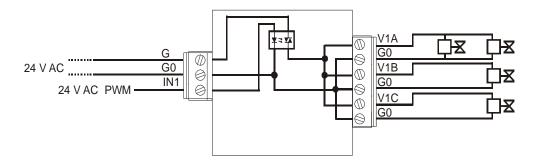
Do not overload the output – maximum triac load is 2 A. Note that the starting currents of cold thermic actuators may be higher than the nominal currents when the body is partially heated.
