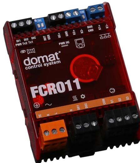
**Summary**                      FCR011 is a 230 VAC powered communicative fan coil controller (up to 3 fan stages, heating and cooling valves). It may either work autonomously or be connected to a primary controller or SCADA. As a room unit, UC010 is used.
