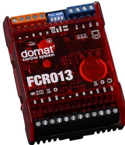
**Summary**      FCR013 is a communicative controller of heating and cooling panels and an EC (electronic commutator) motor or a VAV (variable air volume) damper. It measures room temperature using a room unit and it may either work autonomously, or be connected to a primary controller (markPLC), any other Modbus compatible control system, or SCADA. As a room unit, UC013 is used.
