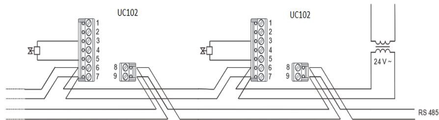
Connection of power, communication, and valve. Suitable cable types are LAM DATAPAR 2×0.8 (cross-section in mm<sup>2</sup>), JYTY 2x1 (diameter in mm) etc. If communication and power are in the same cable, use 4-core LAM DATAPAR 2×2×0.8, JYTY 4×1. Up to 100-120 meters, parallel lines of 24 V and data bus are no problem. Regarding to EMC it is better if the pairs are twisted, such as with the LAM DATAPAR or Belden 8205 cable.
