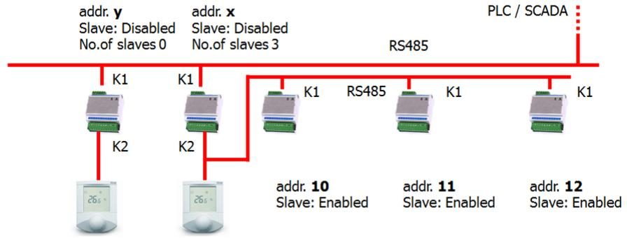
In this connection, controllers with addresses x, 10, 11, and 12 are in one zone and all of them are controlled by one room unit. The controller addressed x is a master. Outputs of controllers addressed 10, 11, and 12 are controlled by the same signals as the master controller addressed x.
