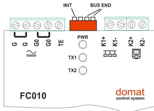
**BUS END:** if ON, the bus is terminated (if last device on the line)
