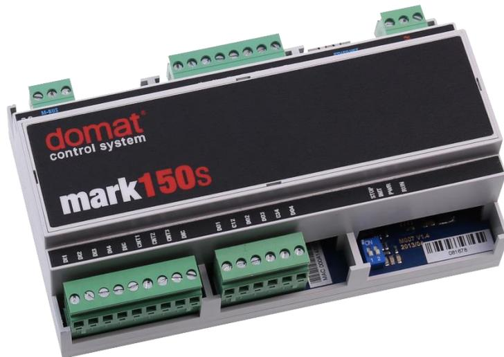
**Summary**      **DDC (Direct digital control) controller mark150s and mark150/485s are free programmable process stations with ARM Cortex M4 processor and OS FreeRTOS. They are suitable for data readout from utility meters or control of small installations (up to about 30 physical data points). They contain 1x Ethernet port, 1x M-Bus interface (maximum 10 meters), 4 AI, 4 DI, 4 DO, and 3 pulse inputs. Mark150/485s contains also 1x RS485 interface.**
