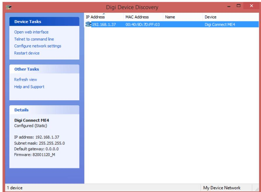
5. In the Device Tasks dialogue set the new IP address (Configure network settings) or go directly to the web pages of the M020 (Open web interface).
