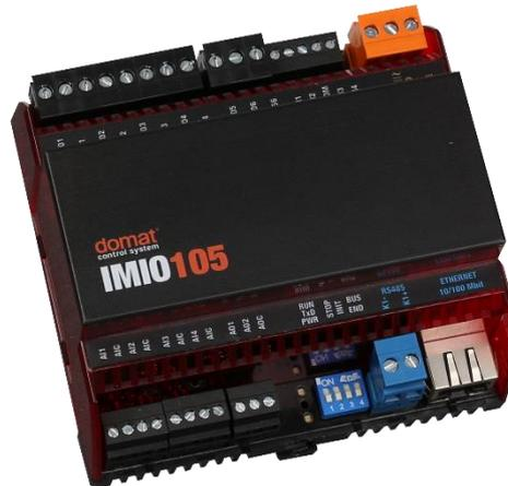
**Summary**      DDC (Direct digital control) controller IMIO105 is free programmable process station with ARM Cortex M4 processor and OS FreeRTOS. It contains one Ethernet port, 4 AI, 4 DI, 2 AO, 6 DO and also a RS485 interface and 8 MB more RAM. IMIO105 is suitable for control of larger installation (approximately 150 physical data points).
