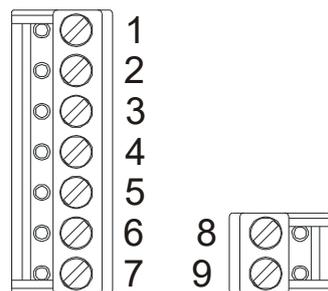
As seen when removing the display part. The wiring goes towards the center of the unit so that the cable can be brought through the aperture in the middle of the bottom part. DI/DO mix is according types, see table below.
