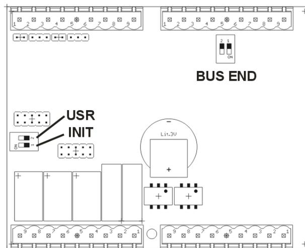
The switches are accessible after the cover is removed.
