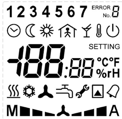
Over Modbus, it is possible to set / reset the complete symbol set except for the 7 segment digits, „Error“ and „Setting“ texts, and symbols of °C, °F, %, and rH. Those are part of the configurable menu profiles. The register description is available in a separate document *Room units UI... – Communication description*. User manual for ModComTool and detailed description of the room unit functions find in the document *Room units configuration – User manual*.
