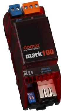
**Summary** DDC (Direct digital control) controller mark100 is free programmable process station with ARM Cortex M4 processor and OS FreeRTOS. It is suitable for control of small installations (up to about 30 physical data points). They contain 1× Ethernet port and 1× RS485 interface. This type is successor of  $\mu$ PLC100. Mark100 dispose with higher RAM memory than  $\mu$ PLC100.
