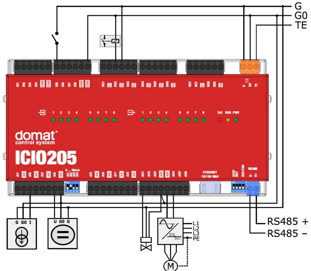
Resistive (passive) sensors are connected between AIx and AIC terminals, for the first 4 inputs must be DIP switch 0...20 mA in the off position. The resistance range is set in the software.
