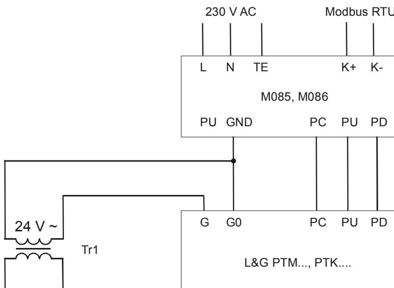
Tr1... original transformer for powering of the I/O
