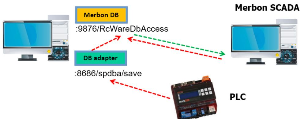
*Flow of history data between a PLC, database, and Merbon SCADA. Red: writing, green: reading.*
